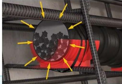
The plastic ducts used in EIT systems provide a shield from corrosive substances and stray currents.
