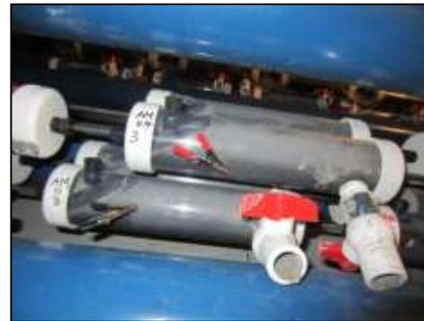
Figure 10. Illustration. Schematic of test specimen containing an artificial void.
